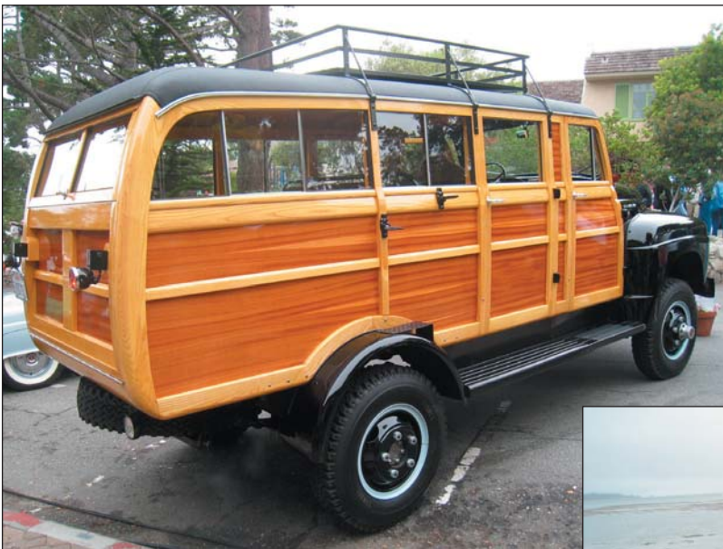
← Carmel's Concours on the Avenue. A 1954 International Harvester 4 WD truck chassis, with a 'woody' body built specifically for National Geographic Magazine
