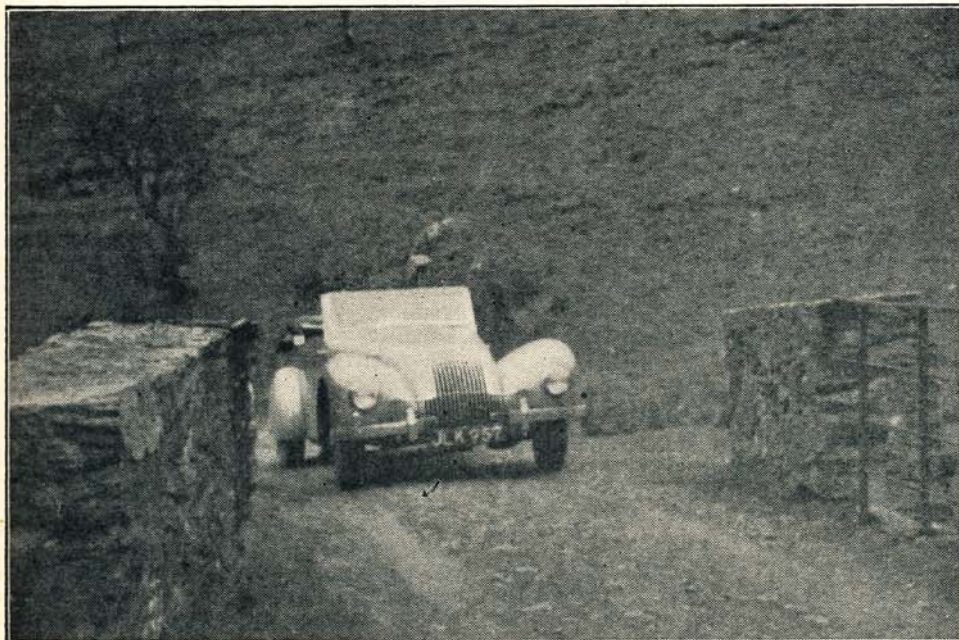
The Allard approaching the rough stuff of North Wales, which it tackled manfully thanks to its 9 in. ground clearance, immense power and good weight distribution.
